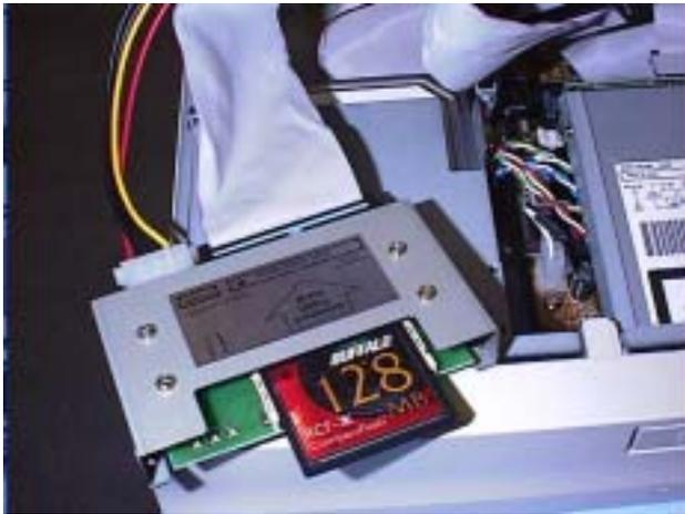
Fig. 4 Compact Flash and IDE interface converter
